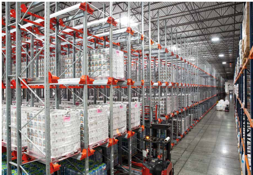
The pallet shuttle system is four levels high and has 74 lanes. It makes fuller use of vertical space compared with floor storage, particularly for loads that don’t stack well.
